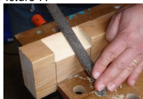
Picture 7 - Removing the last of the excess wood with a rasp file.
