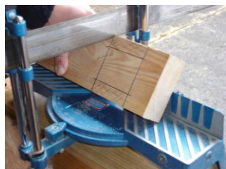
Picture 6 – Cut with either the mitre saw or a Tenon saw like the one shown amongst the tools in Picture 1. The cut is 1.6cm deep on the top edge.
