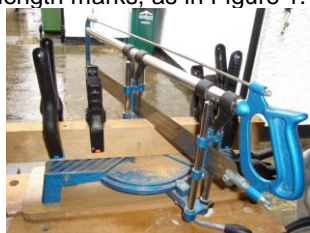
Picture 2-The 1st cut, note the use of clamps to hold the wood in position, there are a couple more holding the Mitre box to the workbench.
