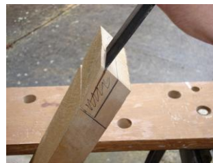
Picture 4 - Remove the waste wood with a chisel (gently does it) cutting away a little at a time. Don't try and chop it all out in one go!
