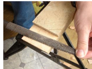
Picture 5 - Removing the last of the excess wood with a rasp file, trim away the rough edges for a smooth finish!
